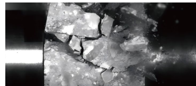
Split Hopkinson Pressure Bar (SHPB)-Versuch
