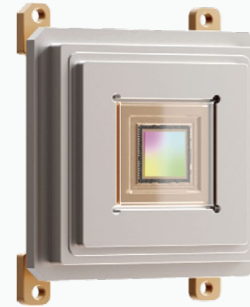
Sealed cavity structure
