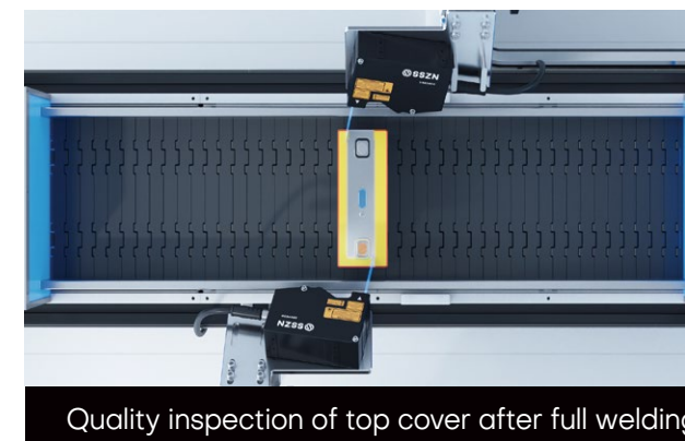
Welding quality inspection of top cap
